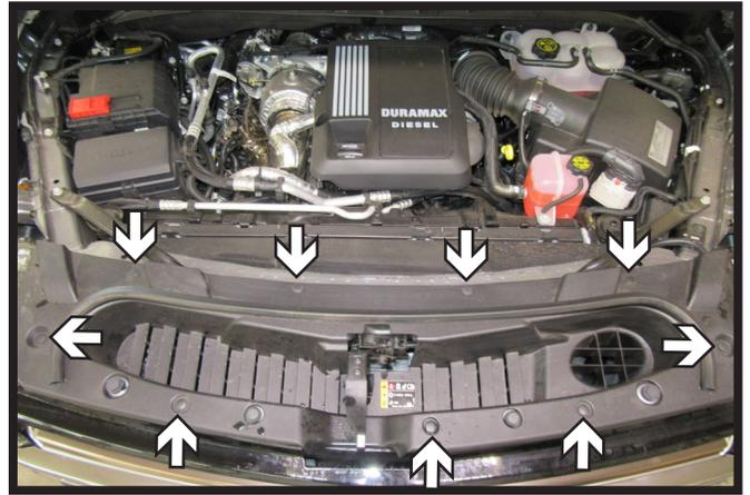
2. Remove the nine (9) push pins from the fascia cover. Remove fascia cover set aside to be re-installed later.
