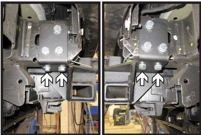
17. Using a 1/2" drill bit, drill the bottom two (2) holes on each side of the vehicle using the baseplate as a template. Then install four (4) 1/2" bolts with lock washers and whiz nuts.
