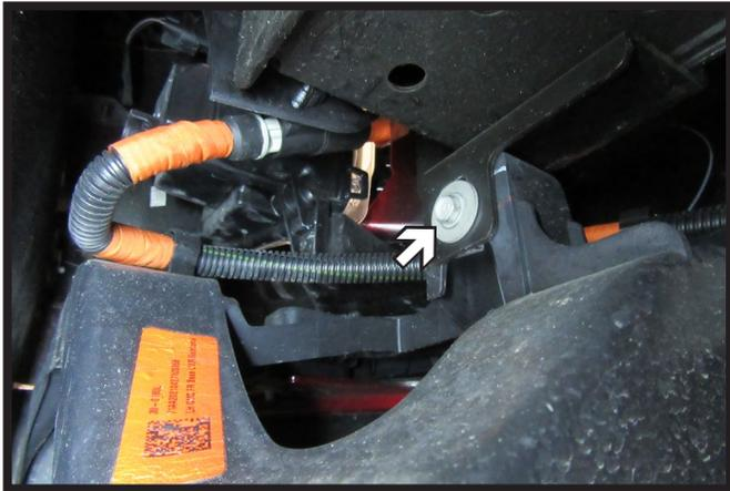
9. **Yukon/Yukon XL Models:** Using a 10MM socket, remove the one (1) bolt on the back side of the fascia in front of the tire. Do this on both sides of the vehicle.
