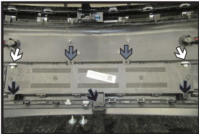
11. **Tahoe Models:** Remove two (2) white clips from cover behind fascia (white). Using a T25 Torx, remove two (2) screws from rear cover (gray). Using a 7MM socket, remove the remaining three (3) bolts from the rear cover (black). Remove cover and set aside. This will not be re-installed.
