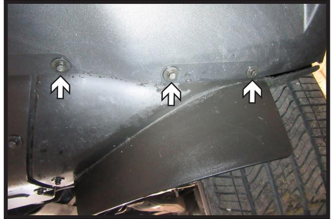
7. Using a 7MM socket, remove the six (6) bolts, three (3) on each side, from the belly pan side covers.
