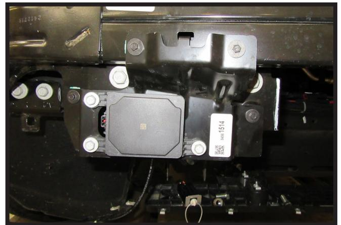
18. **Models With ACC:** Re-install the ACC bracket.
