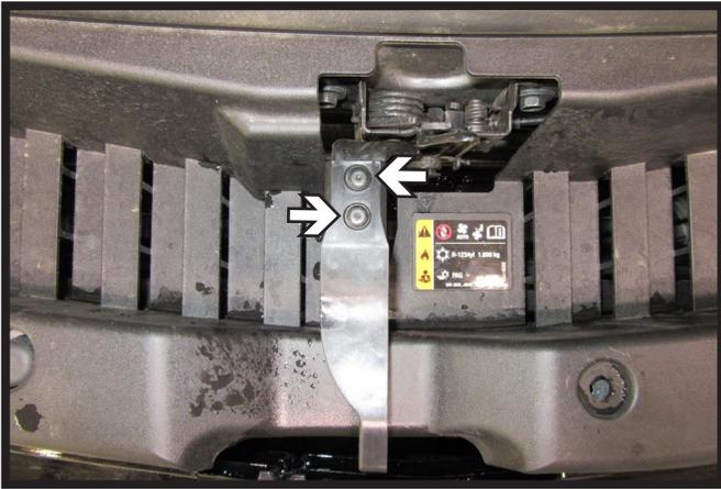
1. Using a T15 Torx, remove the two (2) screws from the hood latch handle. Remove latch handle and set aside to be re-installed later.
