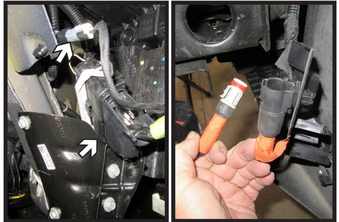
10. ⚠️ Gently pry the fascia loose from the front end. Carefully unplug electrical connections on both sides of the vehicle behind the fascia. Remove the fascia from the vehicle and set aside to be reinstalled later.
