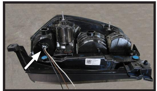
**For BX8869 Only:** Drill a hole according to the tail light wiring kit instructions.
