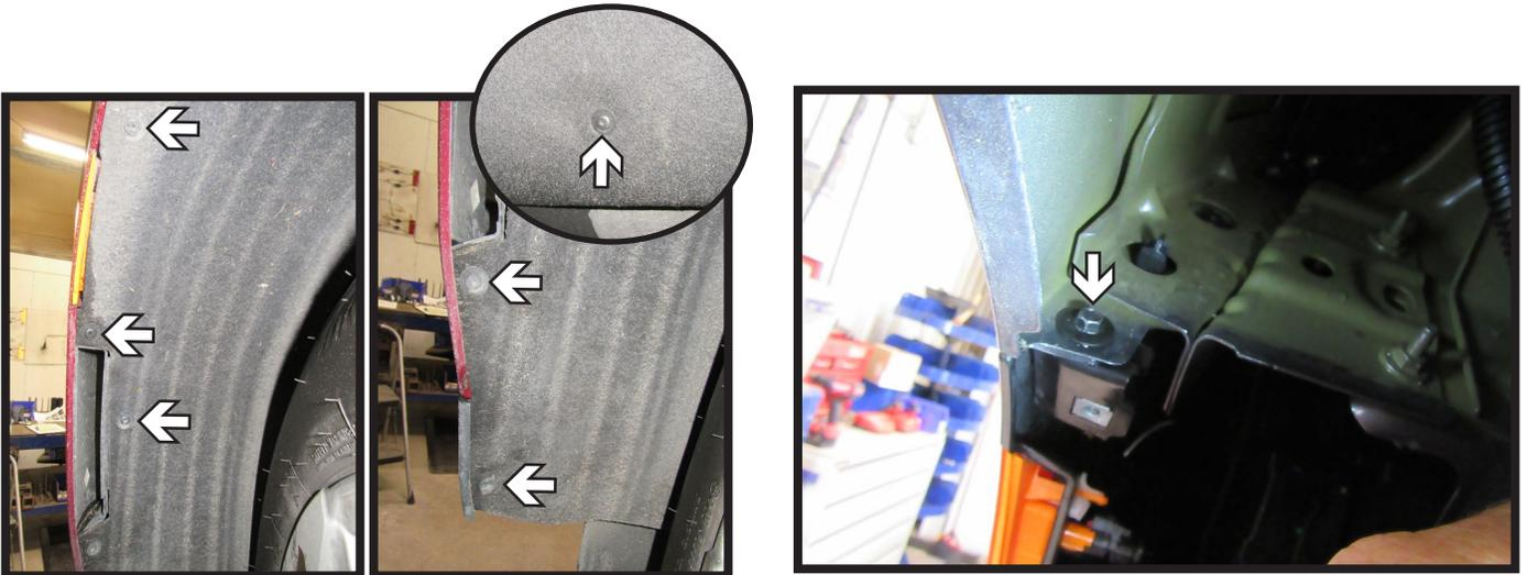
4b. **Yukon/Yukon XL Models:** Using a T15 Torx, remove the six (6) screws from the wheel well liner. Do this on both sides of the vehicle.
