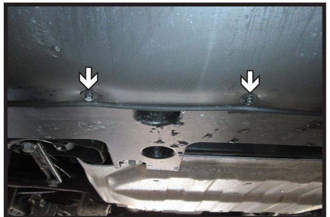
8. Using a 7MM socket, remove the twelve (12) bolts from back of the belly pan, five (5) on each side and two (2) in the middle. Remove belly pan and side covers and set aside to be reinstalled later.
