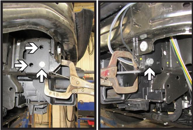
15. Slide the baseplate onto the vehicle and hold in place with vise grips. Install four (4) 1/2" bolts with lock washers and whiz nuts, three (3) bolts on the passenger side and one (1) on the driver side.
