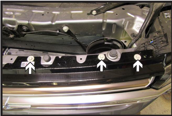
3. Using a 10MM socket, remove the six (6) bolts from top of fascia. There are three (3) on each side of the vehicle.
